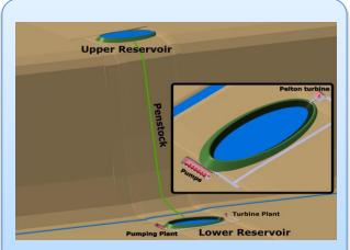
Pumped Storage Plant study under gross head of 770m Plant input/output Electrical Power: 17MW 6 pumps (3MW) & 1 Pelton Turbine (17.7 MW) Location in Alpine Mountain area
